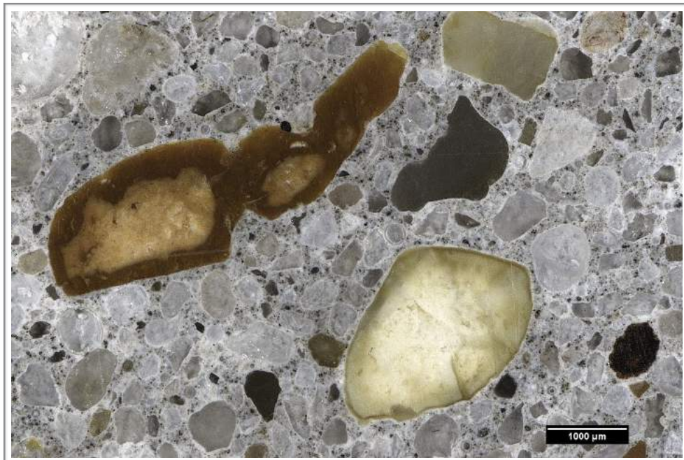
Figure A14. Reflected light photomicrograph of polished surface showing fine aggregate.
