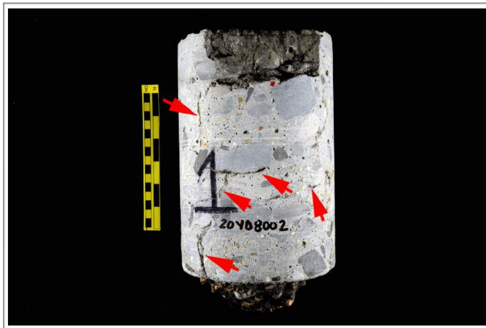
Figure A6. (a) Photograph of the side of the core showing overview of cracks (red arrows). The yellow scale is ~ 150 mm (6 in.) long.
