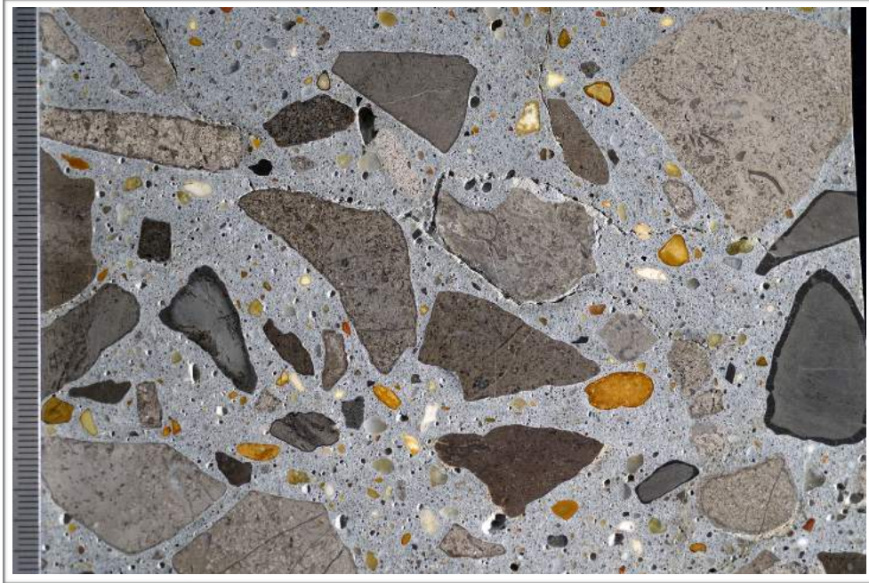
Figure C11. Photograph of polished surface showing overview of coarse aggregate; scale in millimeters.
